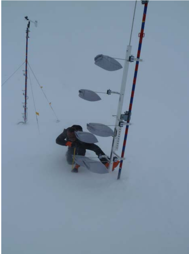
Figure 4: Vertical profile of snow nets used for the measurement of snow concentration in the atmosphere during a blowing snow event.
