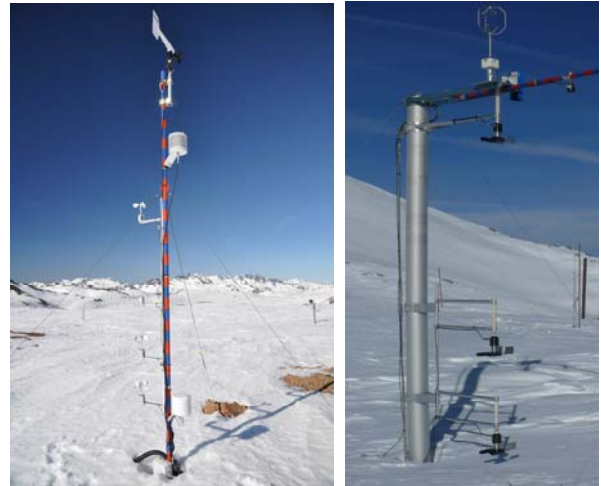
Figure 5: Vertical profile of wind velocity (on the left) and vertical profile of SPC (on the right).
