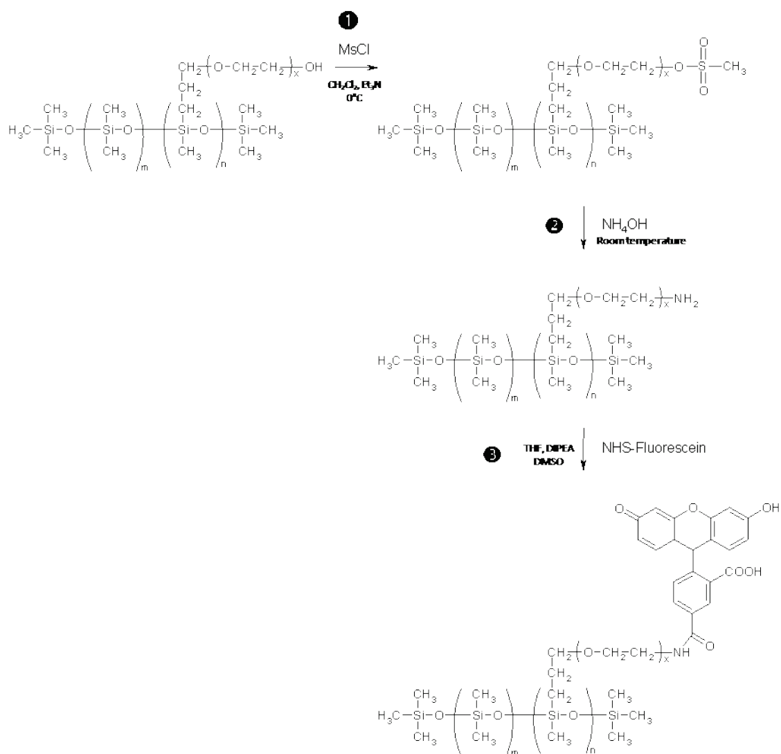
Scheme S-1: Reaction scheme of the tagging procedure of PDMS- g -PEO.
