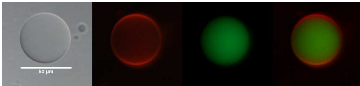
Figure 2. Microscopy acquisitions of a giant polymersome of poly(butadiene)- b -poly(ethylene oxide). From left to right, bright field microscopy, red channel epifluorescence with Nile Red membrane labeling (0.05 mg/mL), green channel with 10.000 g/mol FITC-dextran (1 mg/mL), and overlay of red and green.
