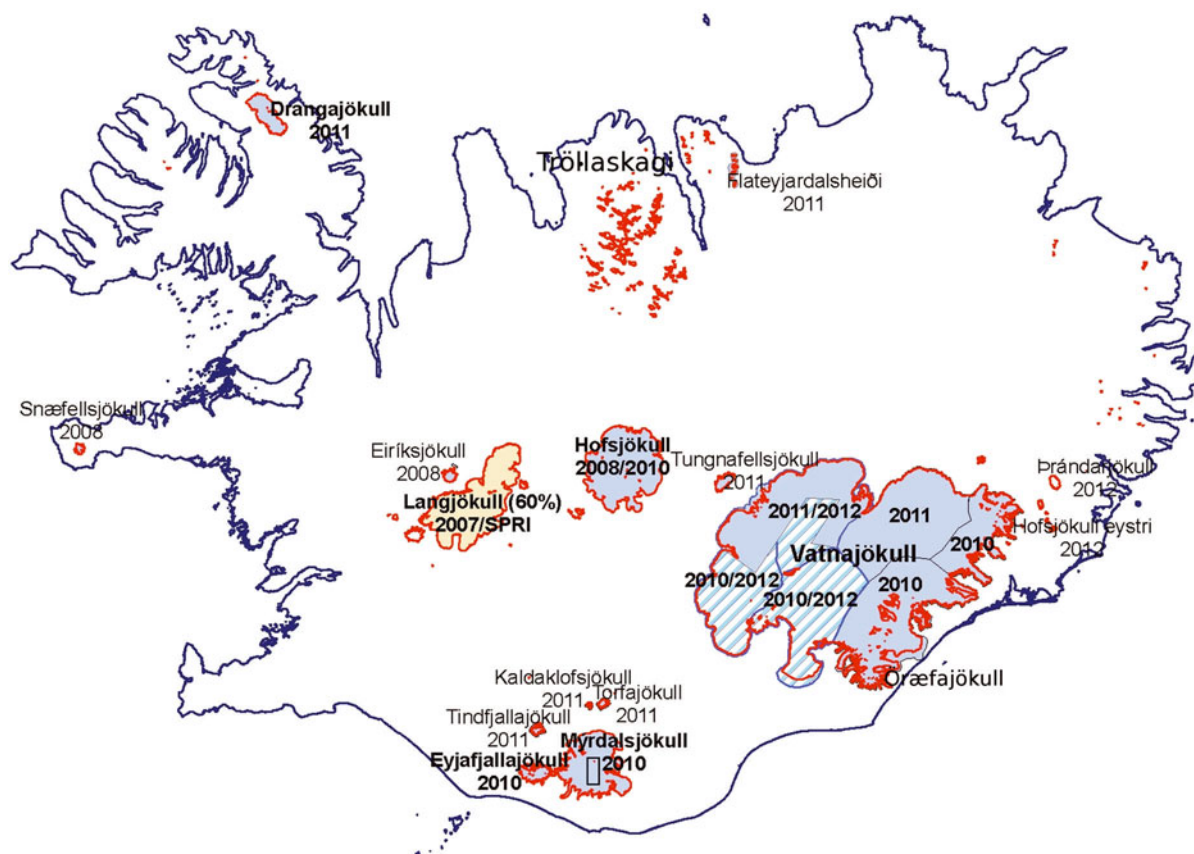
Fig. 1. Location map of Icelandic glaciers showing the status of the lidar mapping at the end of the 2012 surveying effort. Glacier outlines (red curves) were delineated based on orthorectified SPOT5 and Landsat 7 images and aerial photographs from the period 1999–2004. The blue areas were surveyed in 2008–11. Hatched areas on south and southwest Vatnajökull with an area of \sim 2200 \text{ km}^2 were surveyed in 2012 and are being processed. Sixty per cent of Langjökull ice cap (coloured yellow) was surveyed by SPRI in 2007 (Pope and others, 2013). An area on Myrdalsjökull that was resurveyed in 2011 is indicated with a rectangle.
