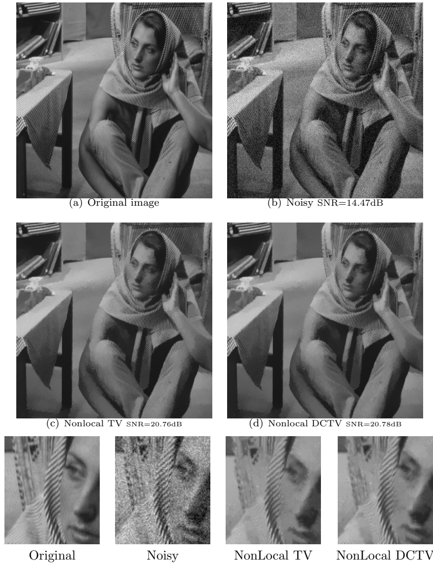
FIG. 3.3. Local and nonlocal denoising (Gaussian noise of variance \sigma^2 = 20 ). The nonlocal weights are computed using [19]. Regularization parameters used to obtain the best results: (e) \lambda = 0.048 (f) \lambda = 0.093 .
