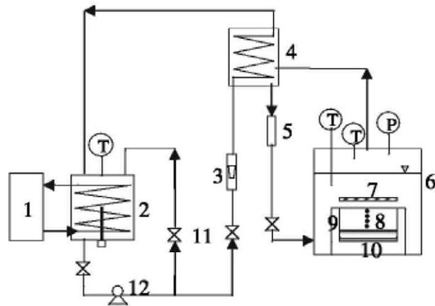
1.R-134a cooling unit 2.Evaporator 3.Water flow meter 4.Condenser 5.Filter/Dryer
