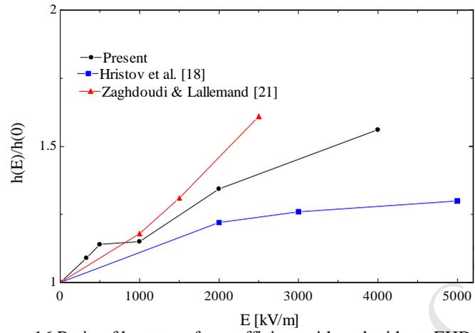
Figure 16 Ratio of heat transfer coefficient with and without EHD at  $100 \text{ kW/m}^2$
