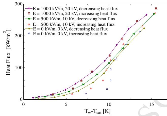
Figure 9 Heat flux verses increasing and decreasing  $\Delta T$
