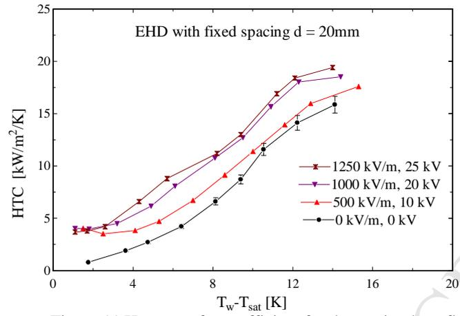
Figure 11 Heat transfer coefficient for decreasing heat flux
