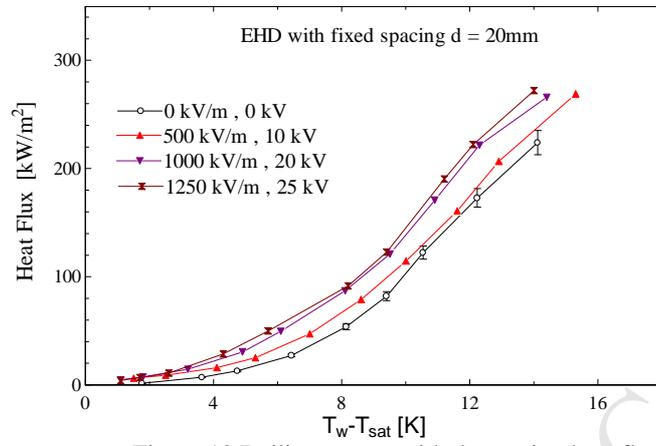
Figure 10 Boiling curves with decreasing heat flux.
