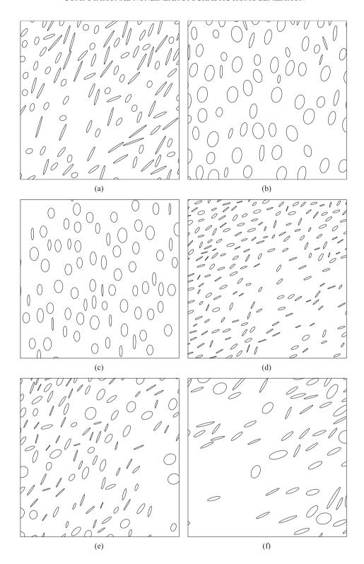
Figure 6. Various geometries of the random microstructure corresponding to different values of input parameters.
