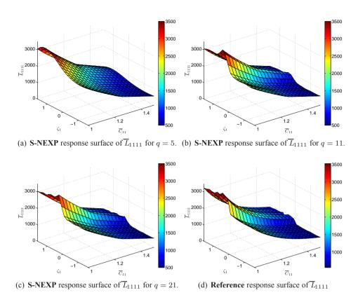
Figure 11. Response surfaces of  $\overline{L}_{1111}$  according to  $\zeta_1$  and macroscopic strains such that  $(\overline{C}_{11}, \overline{C}_{22}, \overline{C}_{12})$  belongs to  $[1, 1.5] \times [1, 1.5] \times [0, 0.5]$  for q = 5, q = 11 and q = 21 and for the reference solution.
