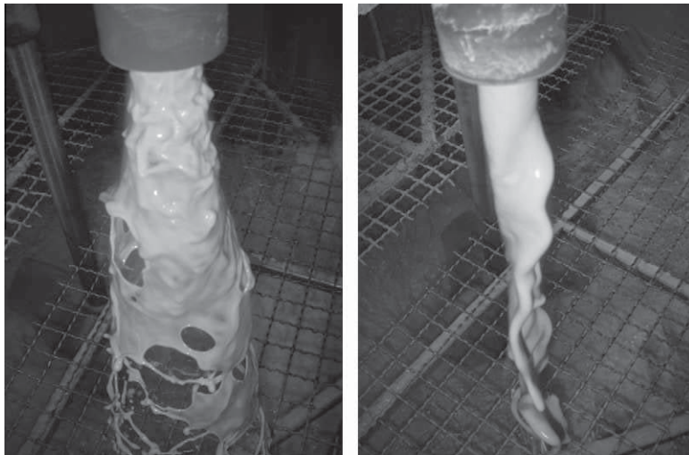
Fig. 7. Photographs of the underflow discharge with feed solid content of 10 wt% and 30 wt%.
