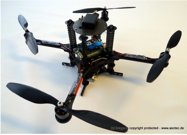
Fig. 8. The Pelican Helicopter used to take inertial data and ground truth data.
