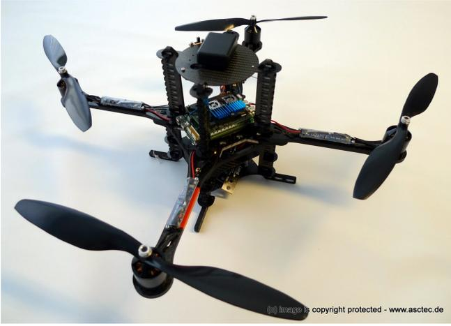
Fig. 8. The Pelican Helicopter used to take inertial data and ground truth data.
