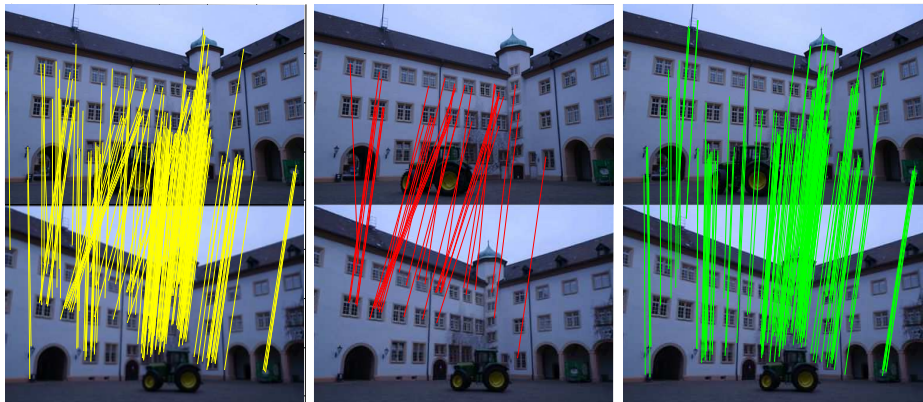
Figure 7: Left: inliers by ORSA. Middle: false matches near epipolar lines not eliminated by ORSA but rejected by K-VLD. Right: inliers by K-VLD + ORSA. (Symmetric matches; Low criterion threshold = 0.8; only 1/4 matches shown, thus matches may show or hide.)
