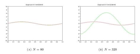
FIGURE 2. Results for N=80 (left) and N=320 (right), using  $P_1$  elements with M=46 in both cases. Instability appears on the right figure.
