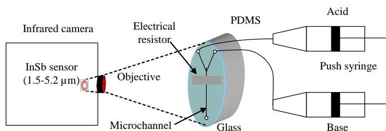
Figure 2: Measurement device
