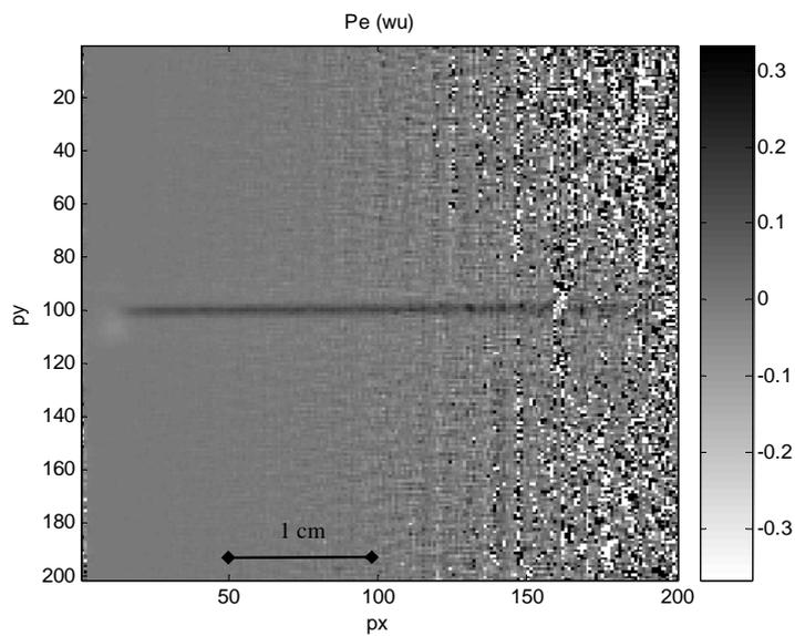
Figure 10-a: Pelet field estimation (global field at 1000  $\mu\text{l/h}$ )
