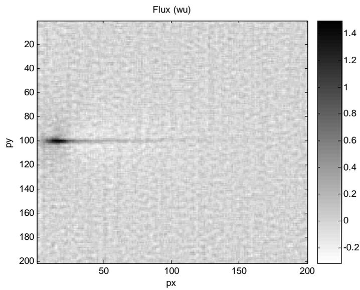
Figure 13-a: Chemical heat source field at 1000  $\mu\text{l/h}$ .
