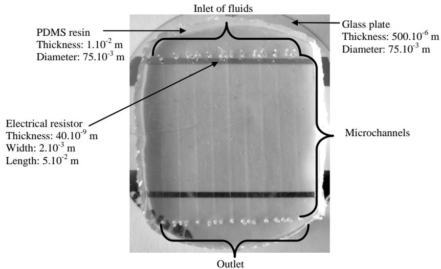
Figure 1: Microfluidic chip, view from the PDMS side.
