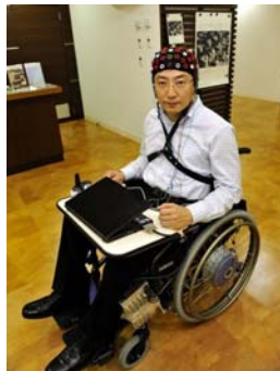
Fig. 7 Toyota wheelchair controlled by BCI [Toyota 2009]
