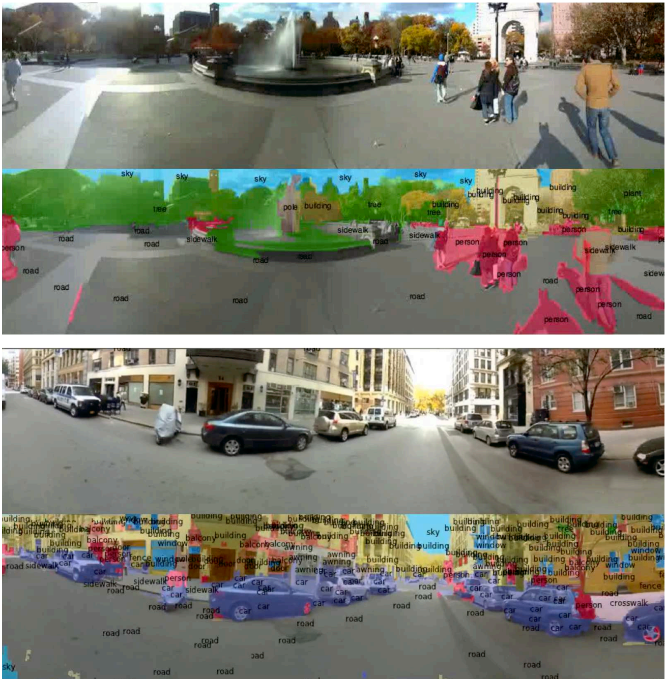
Fig. 11. Real-time scene parsing in natural conditions. Training on SiftFlow dataset. We display one label per component in the final prediction.
