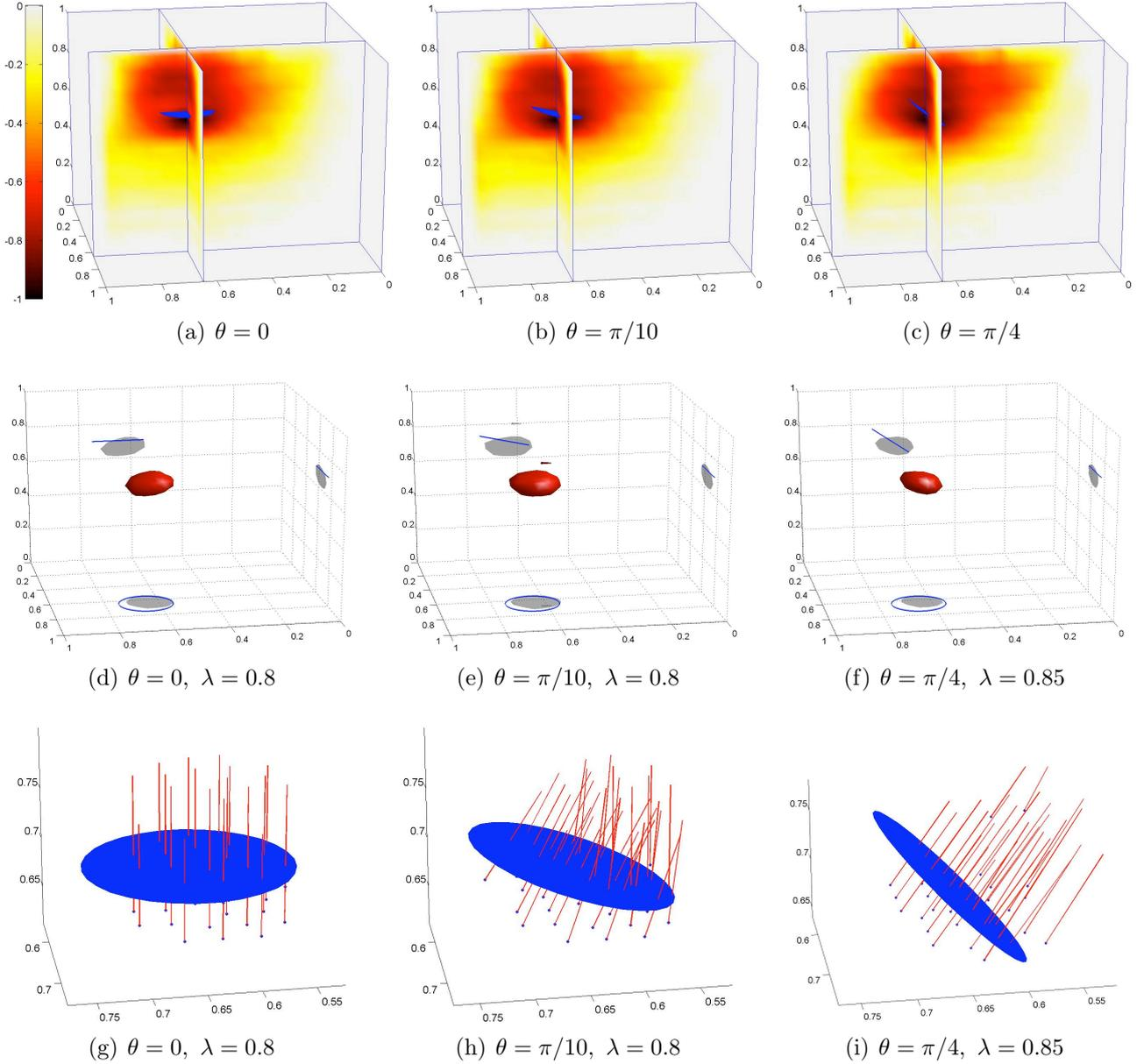
**Figure 3:** Identification of a penny-shaped crack in an elastic unit cube. (a)-(c): normalized TD field  $\hat{\mathbb{T}}_0$ ; (d)-(f): reconstructed domain  $S_\lambda$ ; (g)-(i): optimal normals  $\mathbf{n}_\lambda^{\text{opt}}$  at sampling points
