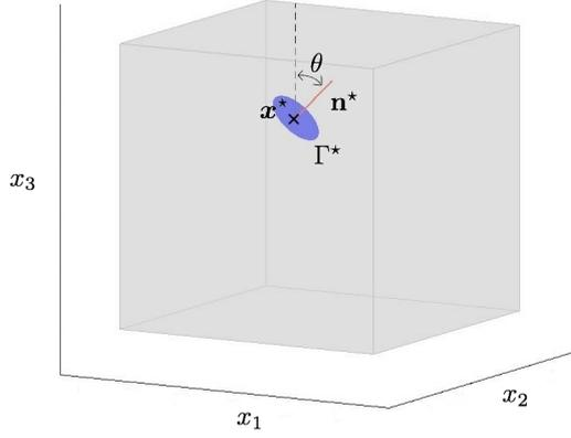
**Figure 1:** Cracked cubic domain
