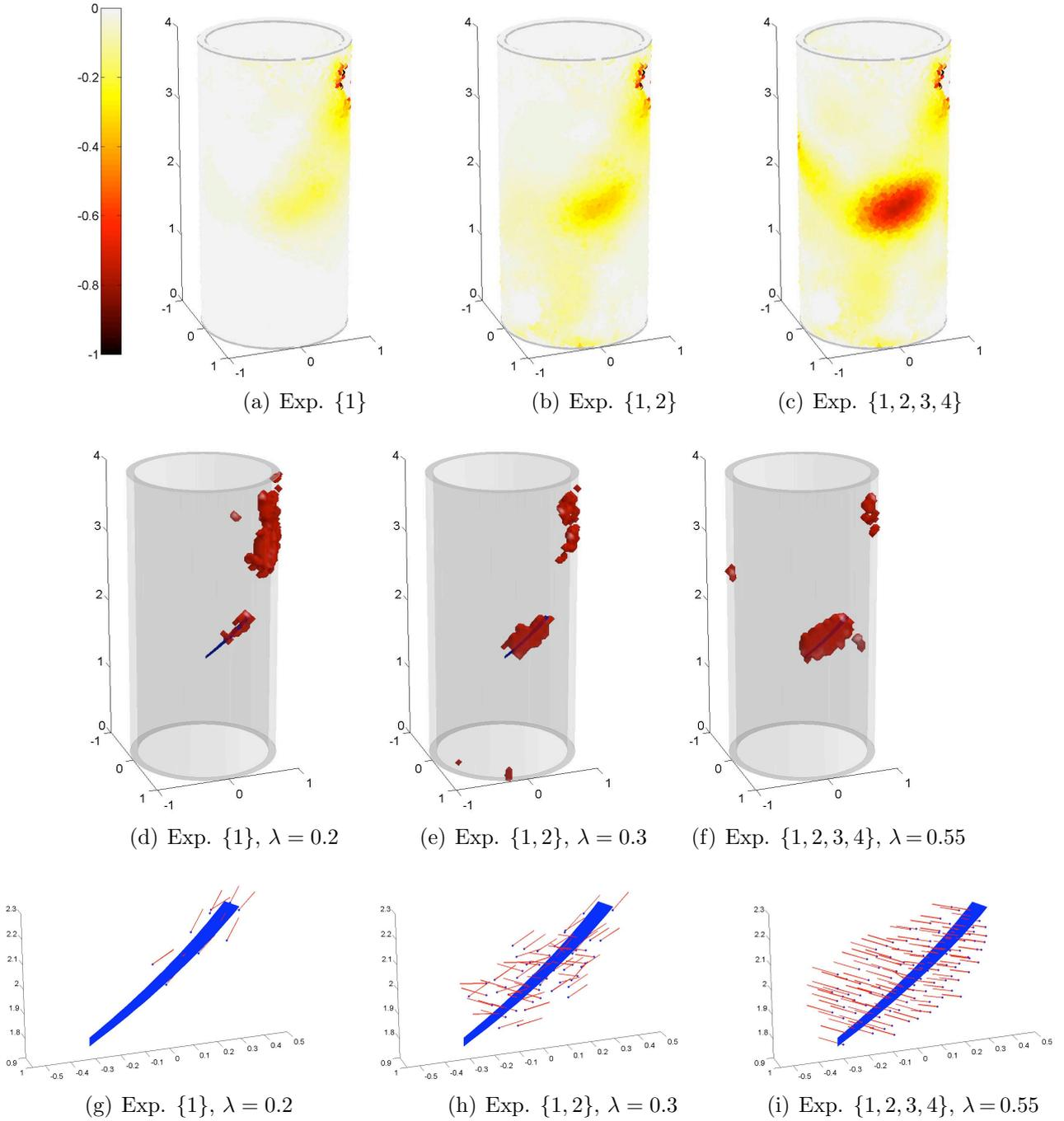
**Figure 7:** Cylindrical shell, cumulated experiments: identification of a single crack. (a)-(c): normalized TD field  $\hat{\mathbb{T}}_0$ ; (d)-(f): reconstructed domain  $S_\lambda$ ; (g)-(i): optimal normals  $\mathbf{n}_{\lambda,0}^{\text{opt}}$  at sampling points
