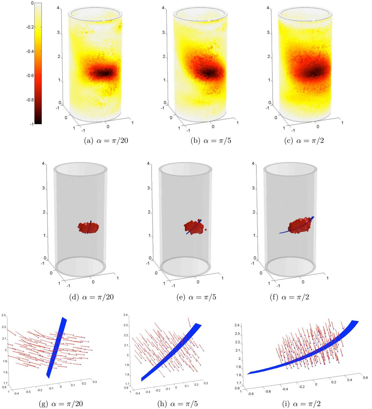
**Figure 5:** Cylindrical shell (elastic), single experiment: identification of a single crack. (a)-(c): normalized TD field  $\hat{\mathbb{T}}_0$ ; (d)-(f): reconstructed domain  $S_{0,8}$ ; (g)-(i): optimal normals  $\mathbf{n}_{0,8,0}^{opt}$  at sampling points
