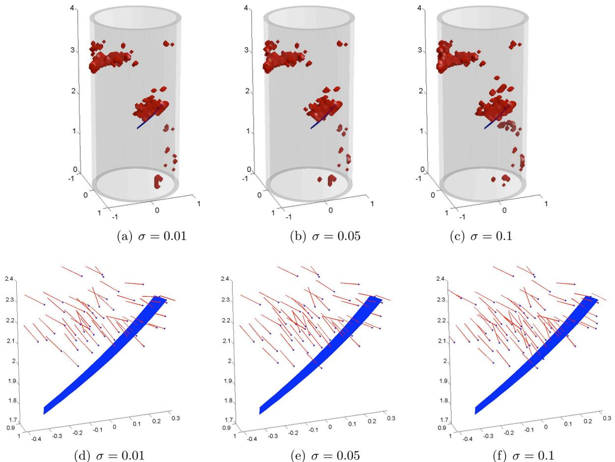
**Figure 6:** Cylindrical shell (elastic), single experiment: identification of a single crack, noisy data. (a)-(c): reconstructed domain  $S_{0.7}$ ; (d)-(f): optimal normals  $\mathbf{n}_{0.7,0}^{\text{opt}}$  at sampling points
