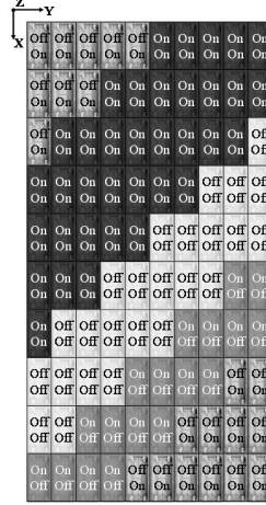
Fig. 7. 10x10 array with a main beam in the (\varphi_{\max} = 45^\circ; \theta_{\max} = 10^\circ) direction
