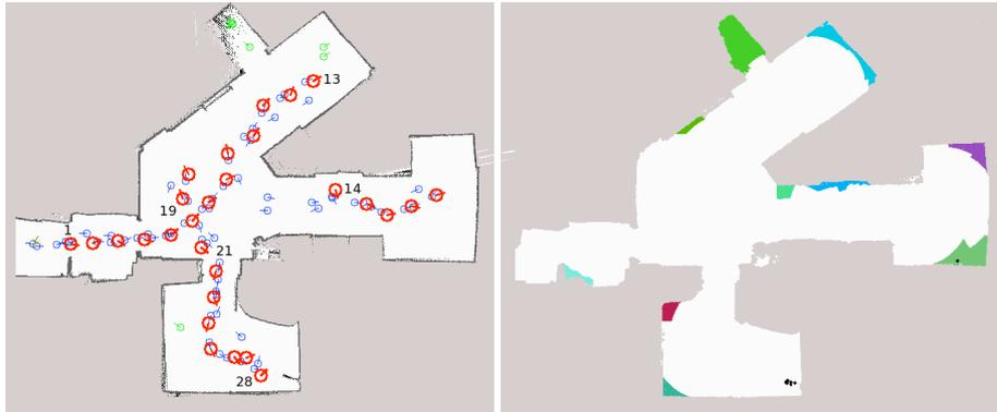
**Fig. 2.** Left: Vision-based exploration map: red circles correspond to exploration points with the robot orientation. Right: view-map showing areas perceived by the camera (*white areas*).
