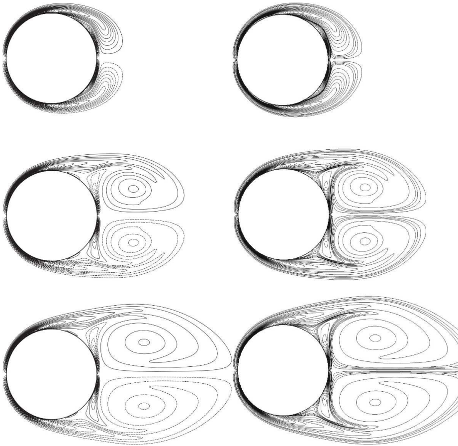
FIGURE 5. Vorticity contours around an impulsively started flow around a circular cylinder for times 1, 3 and 5 (from top to bottom) at Reynolds number 550 (left: vortex-penalization method; right: cut-cell method)
