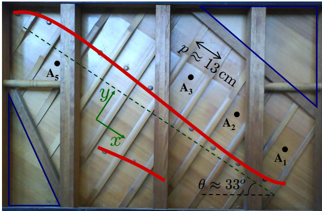
Figure 1: Soundboard of the Atlas upright piano. Rib side with bridges superimposed as thick red lines. This upright soundboard include one ribbed zone and two cut-off corners (blue-delimited lower-left and upper-right triangles).
