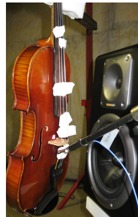
Figure 6: Typical measurement on a violin (in playing conditions, with muted strings) excited by a loudspeaker. The reflective adhesive tape (where the velocity is measured by the laser vibrometer) is visible on the violin soundboard, just above the bridge.
