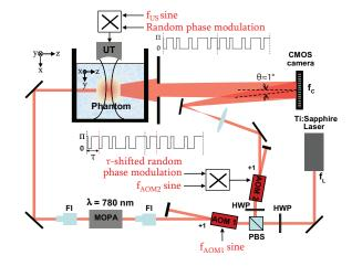
Fig. 1. (Color on-line) Experimental set-up. HWP: half-wave plate, PBS: polarizing beam splitter, AOM1, AOM2: acousto-optic modulators, FI: Faraday isolator, UT: ultrasound transducer,  $f_C$ : camera framerate,  $f_L$ : laser frequency. In the tank, the scheme axes are modified in order to give a view of the inside.
