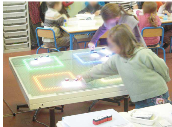
Figure 2: The TangiSense table used in an application to the recognition and learning of colors by children.
