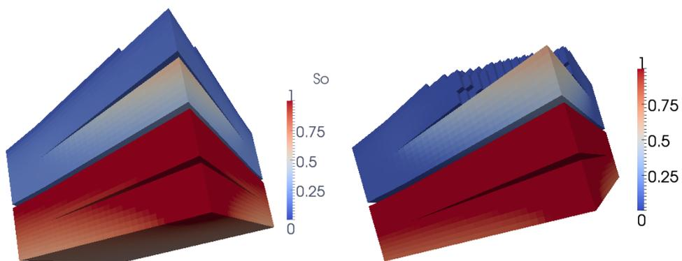
Figure 12: Plot of the oil saturation at final time for  $s_{\mathcal{D}} > 0.05$  computed with the upwind scheme and  $kr_{\min} = 10^{-3} \Rightarrow k_{\min} = 0.2$  (left) and  $kr_{\min} = 10^{-4} \Rightarrow k_{\min} = 0.02$  (right).
