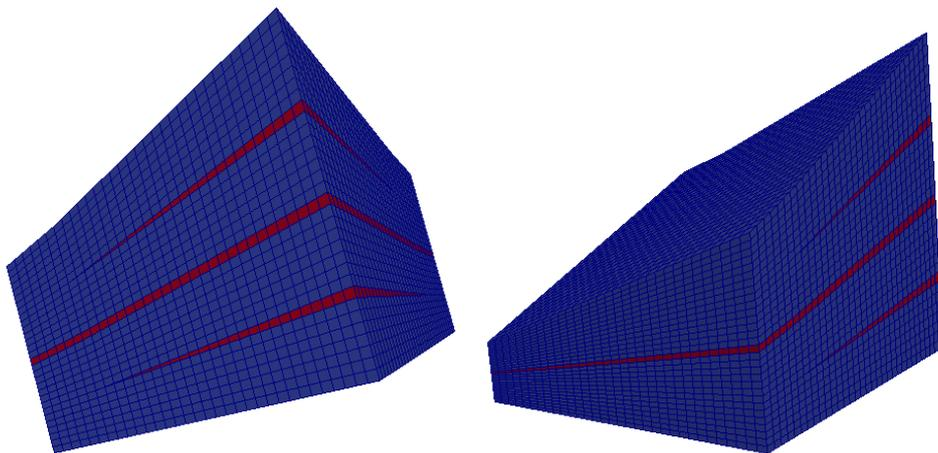
Figure 10: Hexahedral mesh (with degeneracies of some hexahedra due to erosion) of the domain with the three barriers in red (rocktype  $\beta$  in the red barriers and  $\alpha$  outside the barriers).
