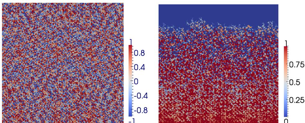
Figure 8: Cellwise constant parameter  $\gamma$  for the rocktype on the triangular mesh with 7297 nodes (left) and discrete oil saturation  $s_{\mathcal{D}}$  computed with the upwind scheme for  $k_{\min} = 0$  with this random capillary pressure.
