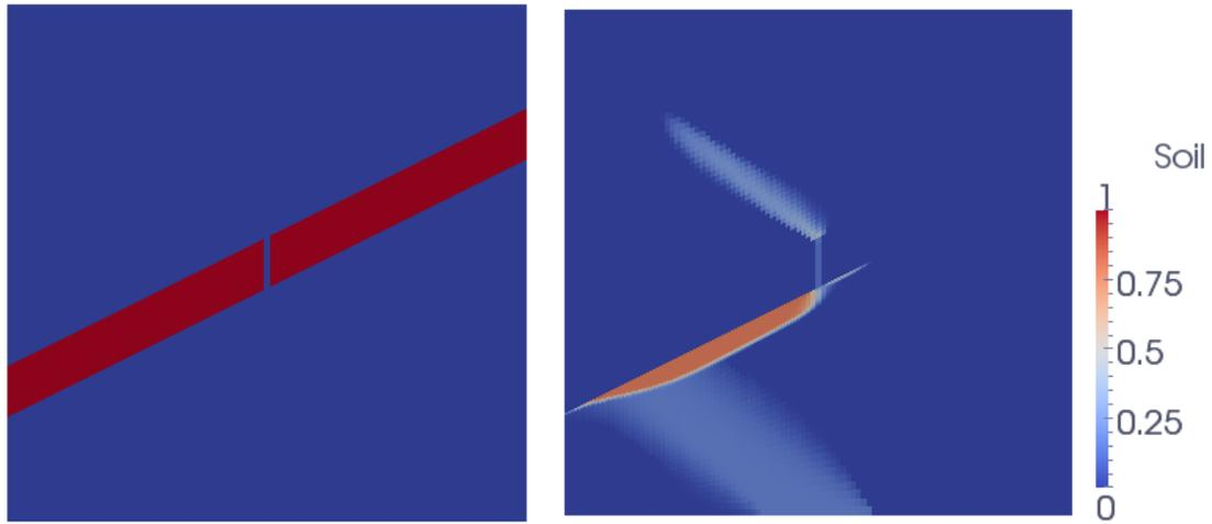
Figure 9: 2D basin with one barrier in red and a fracture crossing the barrier. Oil saturation (phase 1) after 4000 days of simulation on a  $100 \times 100$  quadrangular mesh obtained with the upwind scheme.
