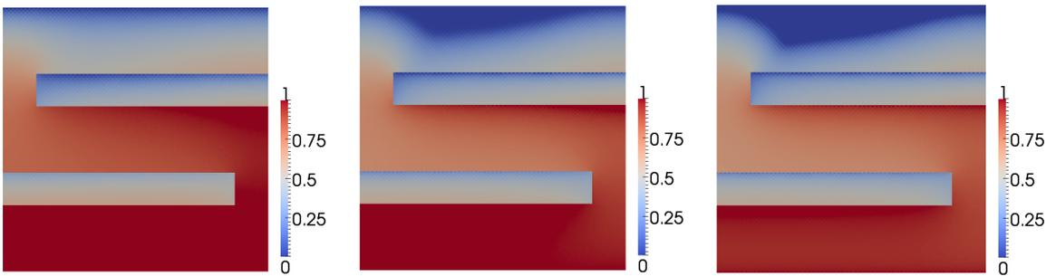
Figure 6: Comparison of the discrete oil saturation  $s_{\mathcal{D}}$  at final time on the uniform Cartesian  $64 \times 64$ , mesh computed with the upwind scheme and different values of  $kr_{\min} = 10^{-1}, 10^{-2}, 10^{-3}$  (which implies here  $k_{\min} = 20, 2, 0.2$ ) from left to right.
