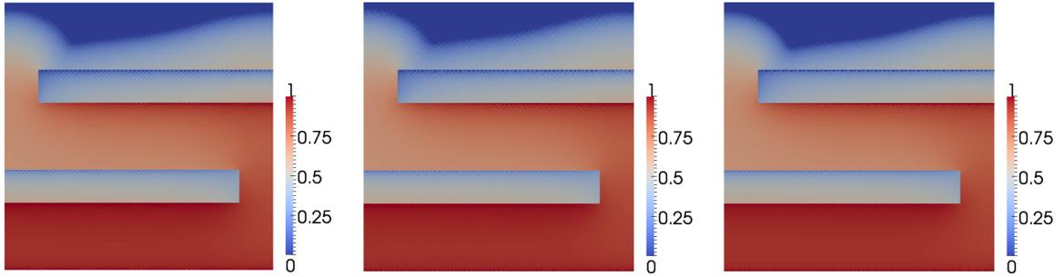
Figure 5: Comparison of the discrete oil saturation  $s_{\mathcal{D}}$  at final time computed with the upwind scheme and  $k_{\min} = 0$  on the uniform Cartesian  $64 \times 64$ , grid, a random quadrangular  $64 \times 64$  mesh, and a triangular mesh with 7297 nodes.
