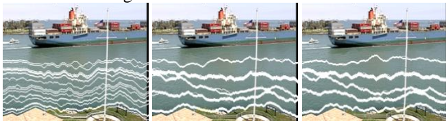
Fig. 5. Seam visible in container. From left to right: Original seams at the encoder, Seams at the decoder with the approach from [2][3] and at the encoder with the closed loop approach, Seams at the decoder with the closed loop approach
