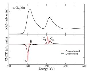
FIG. 6: Calculated (a) XAS and (b) XMCD spectra of  $\alpha$ -Ge<sub>2</sub>Mn at the L<sub>2,3</sub>-edges of Mn. The calculated XMCD spectrum is shown by a thin red line. The same spectrum after convolution with the Lorentzian and Gaussian functions is shown by a thick line. The exchange splitting of Mn 2p core levels was evaluated within the HF approximation.
