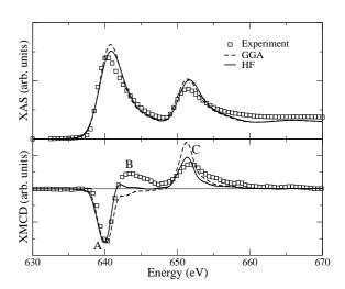
FIG. 4: Calculated (a) XAS and (b) XMCD spectra of  $\rm Ge_3Mn_5$  at the  $\rm L_{2,3}$ -edges of Mn. The exchange splitting of the Mn 2p core levels was evaluated within GGA (dash line) and HF approximation (solid line). Experimental data were taken from Ref. 30.
