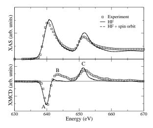
FIG. 5: Calculated (a) XAS and (b) XMCD spectra of  $Ge_3Mn_5$  at the  $L_{2,3}$ -edges of Mn with (dashed line) and without (solid line) spin-orbit interaction. Both spectra are almost superimposed, showing the small influence of the spin-orbit interaction in this metallic compound. The exchange splitting of Mn 2p core levels was evaluated within HF approximation.
