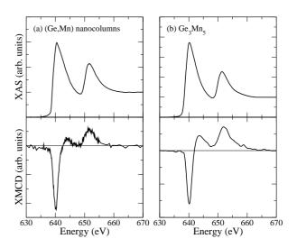
FIG. 1: (a) Experimental XAS and XMCD spectra in the (Ge,Mn) nanocolumns measured at a temperature of 5 K and in a 5 T magnetic field and (b) in  $Ge_3Mn_5$  at 80 K and in remanence (from Ref. 30).
