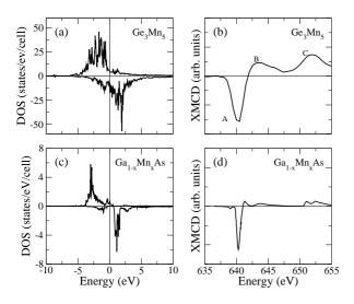
FIG. 3: 3d-states of Mn in (a)  $Ge_3Mn_5$  and (c)  $Ga_{1-x}Mn_xAs$  (x=0.125). Experimental XMCD spectra at the  $L_{2,3}$  edges of Mn in (b)  $Ge_3Mn_5$  (from Ref. 30) and (d)  $Ga_{1-x}Mn_xAs$  (x=0.084, from Ref. 31).
