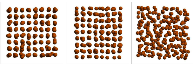
Figure 5. (Color online) Instantaneous pictures of the supercell of Ar for different temperatures, respectively from left to right : 75 K (far below T_m ), 92 K (close to T_m ) and 100 K (above T_m ).
