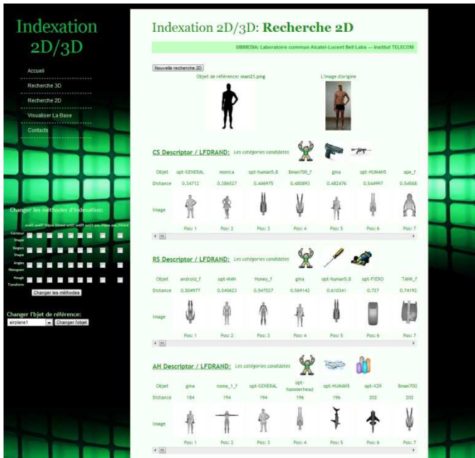
Figure 6. 2D/3D retrieval and categorization with the proposed system, with a query representing a humanoid.
