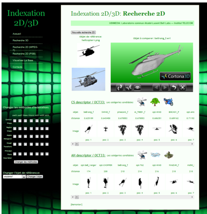
Figure 7. 2D/3D retrieval and classification with the proposed system. Upper images represent the query object segmented from the image and the original image. Lower, we can observe the views of the 3D models retrieved in first positions. For each 2D/3D indexing method the three most probable categories are illustrated by the three icons (in this example a helicopter, a tank and a motorcycle for the CS descriptor and a helicopter, an airplane and a tank for the AH descriptor).
