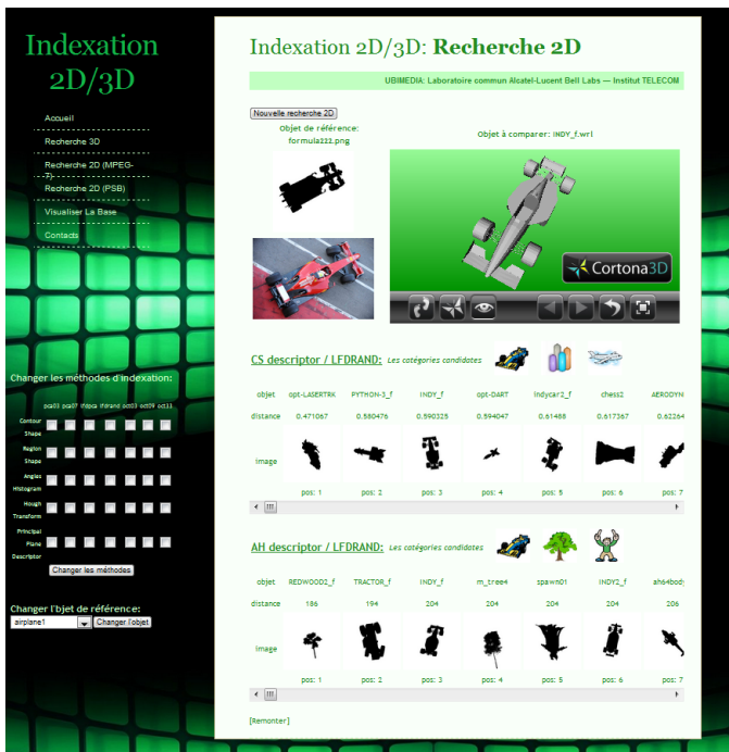
Figure 8. 2D/3D retrieval and classification with the proposed system. Query representing a formula 1 car.
