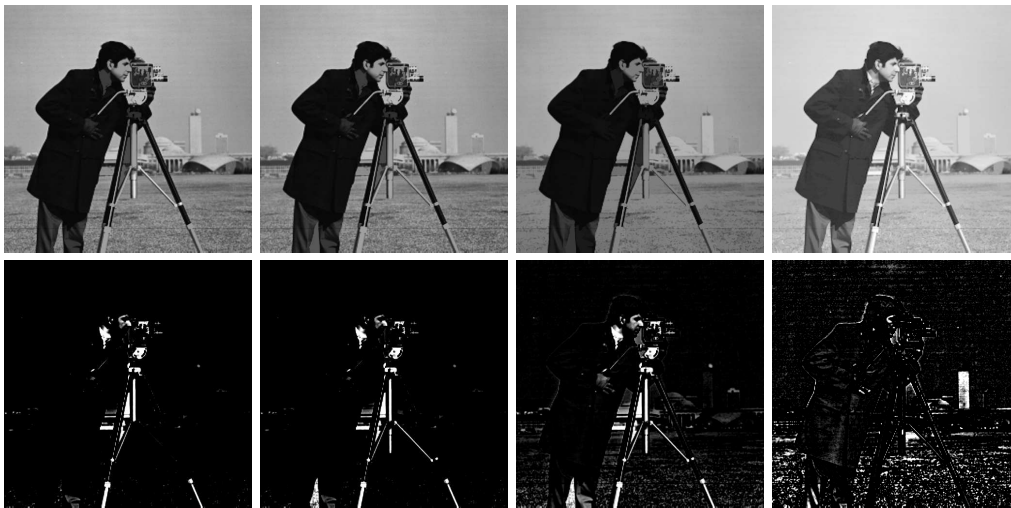
Figure 9. Connected filtering of the traditional camera image. The first row shows the results of the filters and the second row shows the difference with the original image (contrast increased). From left to right: area filter (1000 pixels) based on the h-component tree with the fuzzy h-connection C_{f,0.8}^+ , area filter (1000 pixels) using the k-zone reconstruction method [23], [24] ( k=0.2 ), area filter (1000 pixels) using traditional Max-Tree [5] and dynamic opening proposed in [33]. The results show that both the h-component tree and the k-zone approach lead to a better preservation of textures. The proposed approach concentrates only on distinct zones with sufficient contrast, while internal details of objects, textures, and softly connected objects are preserved.
