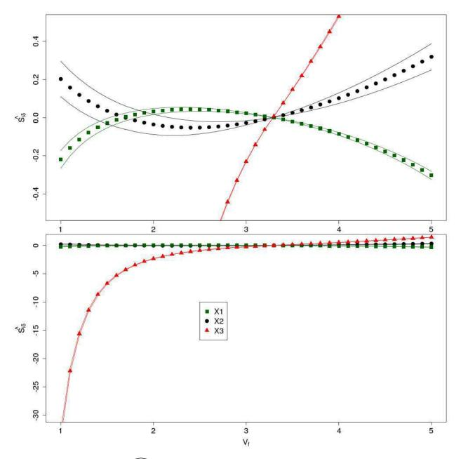
Figure 6: Estimated indices  $\widehat{S_{i,V_{\mathrm{per}}}}$  for the thresholded Ishigami function with a variance shifting. The upper figure is a zoom where the  $\widehat{S_{i,V_{\mathrm{per}}}}$  axis lies into [-0.5,0.5]. The lower figure shows almost the whole range variation for  $\widehat{S_{i,V_{\mathrm{per}}}}$ . The curves cross for the value of  $V_{\mathrm{per}}$  that corresponds to the original variance, namely  $\pi^2/2$
