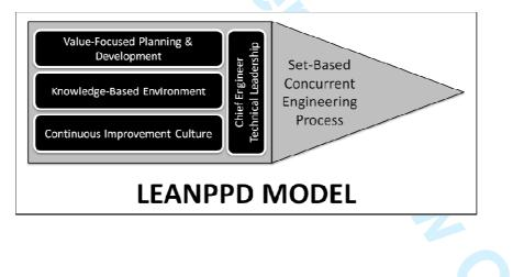
Figure 3- Set-based concurrent engineering process
