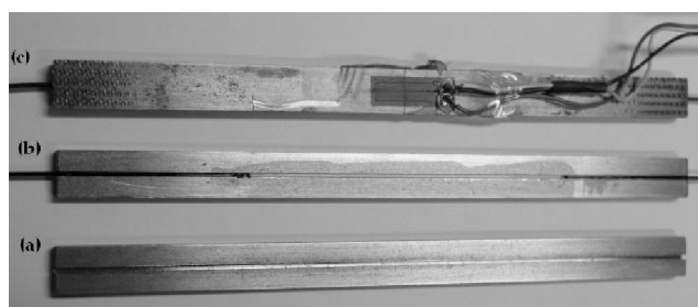
Figure 6. Metallic specimen naked (a), with Fibre sensor embedded ((b) and (c)) with a strain gauge sticks on the opposite side (c)
