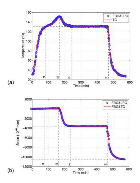
Fig. 2. Temperature (a) and strain (b) measured with the superimposed LPG/FBG sensor during the curing process.
