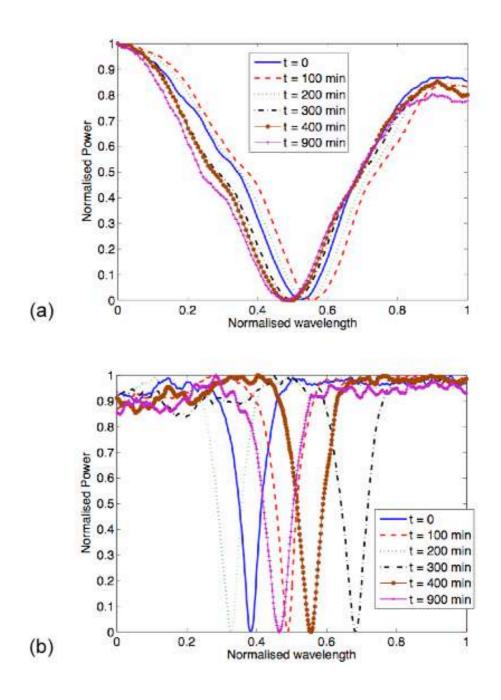
Fig. 7. LPG spectra (a) and FBG spectra (b) at several times during the LRI process.
