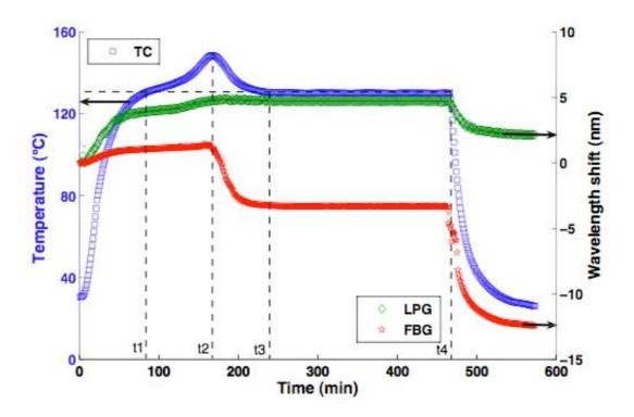
Fig. 1. Thermocouple temperature (left), FBG and LPG wavelength shifts (right) vs. time recorded for the temperature cycle applied to the resin sample.
