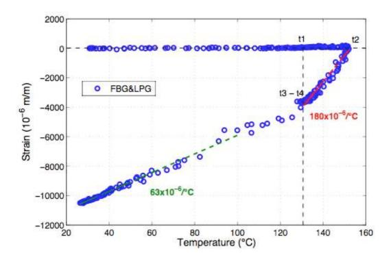
Fig. 3. Strain versus temperature measured by the FBG/LPG sensor during the curing of the epoxy resin.
