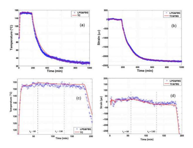
Fig. 6. Temperature (a) and strain (b) measured with the superimposed LPG/FBG sensor during the LRI process. (c) and (d) are respectively the enlargement of (a) and (b).
