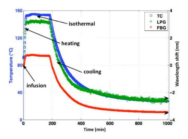
Fig. 4. Thermocouple temperature (left), LPG and FBG wavelength shifts (right) during the LRI process.
