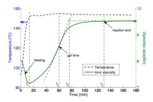
Fig. 5. Measurement of the resin ionic viscosity with DEA system during the first two phases (heating and isothermal plateau) of the LRI process.
