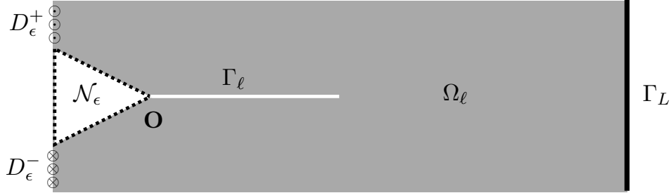
FIGURE 3. The cracked notch-shaped body \Omega_\ell
