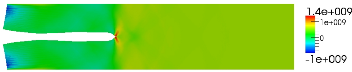
Fig. 12 Mode I fracture. Deformed configuration (enlarged 50 times) and stress \sigma_{yy} at time T . Scheme B ( n_{mesh} = 800 , \nu_C = 1 ).
