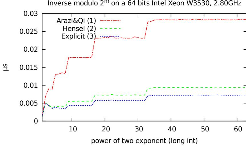
Figure 1: Modular inverse on 64 bits machine words
