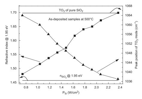
Fig. 1. Evolution of the refractive index n taken at 1.95 eV energy (left axis) and of the TO<sub>3</sub> Si-O peak position (right axis) versus  $P_{Si}$  for as-deposited samples. The lines on top and bottom are the TO<sub>3</sub> position (1065 cm<sup>-1</sup>) and the refractive index n (1.457) for pure SiO<sub>2</sub> grown at the same conditions with the same thickness as SRSO-Nd layers, respectively.
