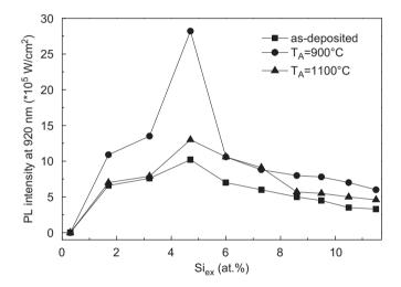
**Fig. 5.** Evolution of the  $Nd^3$  + PL intensity at 920 nm as a function of the  $P_{Si}$  for as-deposited and annealed films.
