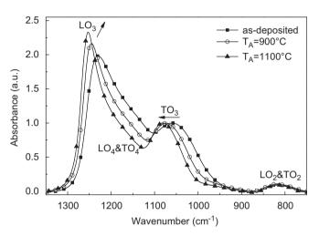
Fig. 3. Typical evolution of the FTIR spectra measured in Brewster incidence for as-deposited and annealed films.
