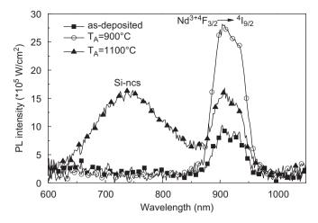
**Fig. 4.** Typical evolution of the PL spectra of sample with  $P_{Si}$ =1.33 W/cm<sup>2</sup> for as-deposited and annealed films.
