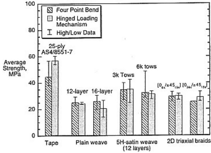
Figure 13 Out-of-plane tensile strength of different material systems.
