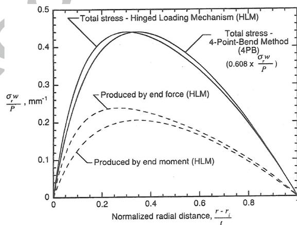
*Figure 12 Stress distributions in the L-shaped flexural specimens*
