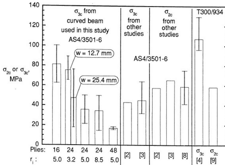
Figure 14 Geometry influence on transverse tensile strength.
