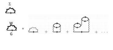
**Fig. 2**. The self-energy in a generally accepted approximation is represented by a propagator G multiplied by the interaction W and integrated over internal exchanged momentum. The effect of potential screening can be visualized as a summation over infinite ladder contributions.
