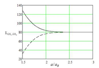
**Fig.5**. GS energy level splitting by effect of QD-QD coupling, for two stacked layers of self-assembled InAs/GaAs quantum dots, at null carrier density. Electron mass *m* has been set to 0.060 free electron mass. In abscissas,  $a/a_B$  is the layers separation in unit of Bohr radius  $\hbar/\sqrt{m \ \tilde{\epsilon}_{GS}}$  (here  $\approx 4 \text{ nm}$ ).
