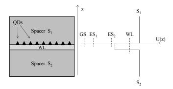
Fig. 1. On the left, a sketch of a WL-QD layer grown by Stranski-Krastanow method is shown. On the right, conduction band is shown with the confining potential U(z), the WL bound level (substantially a very thin quantum well), ground state (GS) and excited states (ES) of quantum dot.
