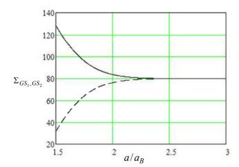
Fig.5. GS energy level splitting by effect of QD-QD coupling, for two stacked layers of self-assembled InAs/GaAs quantum dots, at null carrier density. Electron mass m has been set to 0.060 free electron mass. In abscissas,  $a/a_B$  is the layers separation in unit of Bohr radius  $\hbar/\sqrt{m\ \breve{\epsilon}_{GS}}$  (here  $\approx 4$  nm).
