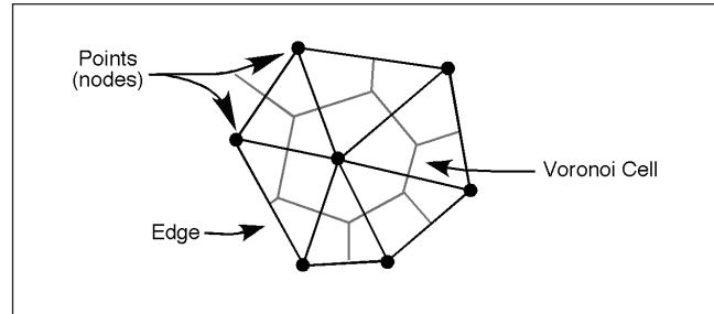
**Fig. 2 – Schematic illustration of the spatial framework in CHILD model.** The study area ( $16 \text{ km}^2$ ) is discretized into 40000 Voronoï cells. Each cell is  $400 \text{ m}^2$  large.
