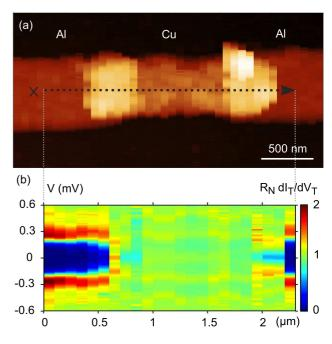
FIG. 4: Typical measurements obtained with our cryogenic AFM/STM on a hybrid Josephson junction at 90 mK. a) AFM image of the Al/Cu/Al junction. The cross indicates where spectroscopies in out-of-equilibrium conditions were realized, see Fig. 5b. b) Color plot of local spectroscopic data  $dI_T/dV_T(V_T)$  performed every 100 nm along the dotted arrow with a tunnel resistance of 10 M $\Omega$ .
