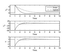
Fig. 5. Hybrid and linear controllers for  $\alpha = 2$  (zero initial condition).
