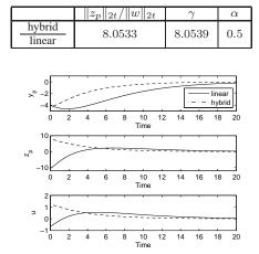
Fig. 2. Hybrid and linear controllers for  $\alpha = 0.5$  (no disturbance).
