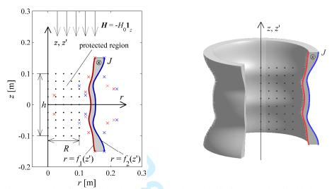
Figure 1. a) On the left - a definition sketch for an exemplary solenoid with protected region (black dots);  $x, x - f_1$  and  $f_2$  Bezier curves' control points; b) on the right - 3D visualization.
