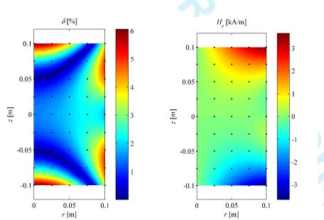
Figure 6. a) On the left - relative error  $\delta$  [%] for desired ( $H_0 = 45$  kA/m) and calculated magnetic field; b) on the right - distribution for the magnetic field radial component  $H_r$  [kA/m].
