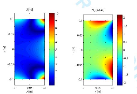
Figure 8. a) On the left - relative error  $\delta$  [%] for desired ( $H_0 = 55$  kA/m) and calculated magnetic field; b) on the right - distribution for the magnetic field radial component  $H_r$  [kA/m].
