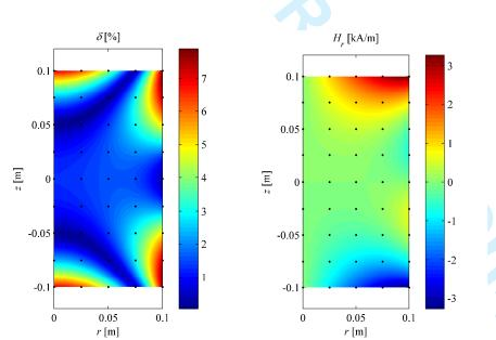
Figure 4. a) On the left - relative error  $\delta$  [%] for desired ( $H_0 = 35$  kA/m) and calculated magnetic field; b) on the right - distribution for the magnetic field radial component  $H_r$  [kA/m].
