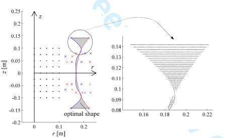
Figure 11. a) On the left - optimal shape of the solenoid for desired  $H_0 = 45$  kA/m; b) on the right - magnified upper part of the solenoid; black points represent middle of the wires with current equal to 10 A.
