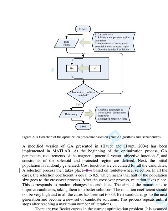
There are two Bezier curves in the current optimization problem. It is assumed that each Bezier curve is built from six control points  $C_i$  ( $r_i$ ,  $z_i$ ), i = 0, 1, 2, 3, 4, 5. ThisIt means that the total number of optimized parameters is equal to 24. Possible values (the search space) of the parameters for the  $f_1$  curve and  $f_2$  curve are the same and have been shown in Table. 1. The population size was equal to 32, and the total number of generations was equal to 500.
