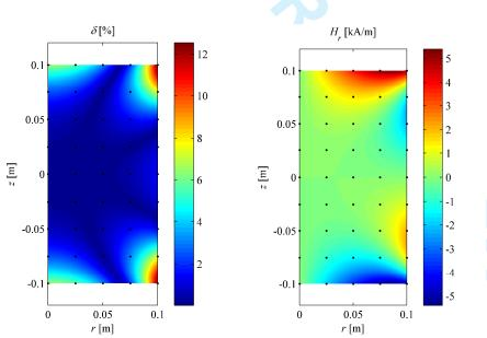
Figure 10. a) On the left - relative error  $\delta$  [%] for desired ( $H_0 = 70$  kA/m) and calculated magnetic field; b) on the right - distribution for the magnetic field radial component  $H_r$  [kA/m].
