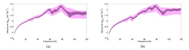
Figure 6: Modulus, in log scale, of the random frequency response function for  $Ob_{4}$  (a) et  $Ob_{2}$  (b). Confidence region (dark gray region) computed with the reference computational model. Confidence region (magenta region) computed with the stochatic reduced-order model. Deterministic response calculate the elastic modes (black solid thick line)
