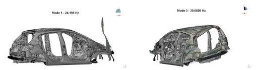
Figure 3: First elastic mode (left) and third elastic mode (right).
