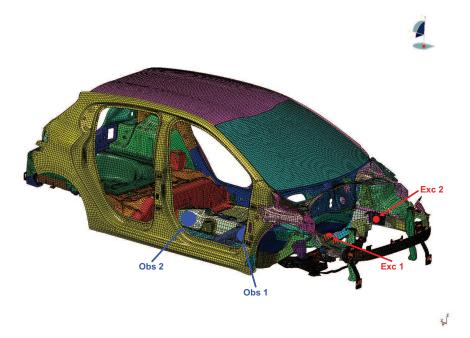
Figure 1: The Finite Element model of an automotive vehicule
