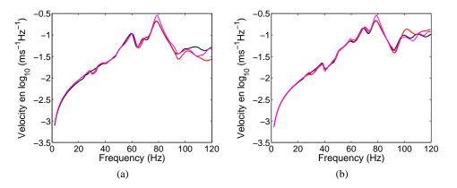
Figure 5: Modulus, in log scale, of the frequency response function for  $Obs_1$  (a) and  $Obs_2$  (b). Comparisons between different projection bases: elastic modes (black solid thick line), global displacements eigenvectors only (red solid thick line), global displacements eigenvectors with modification of the damping matrix (magenta solid thick line), global and local displacements eigenvectors (solid thin line superimposed to the solid thick line).
