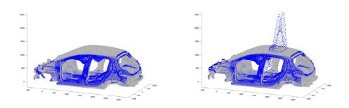
Figure 4: Fourth global displacements eigenvector (left) and corresponding eleventh elastic mode (right).
