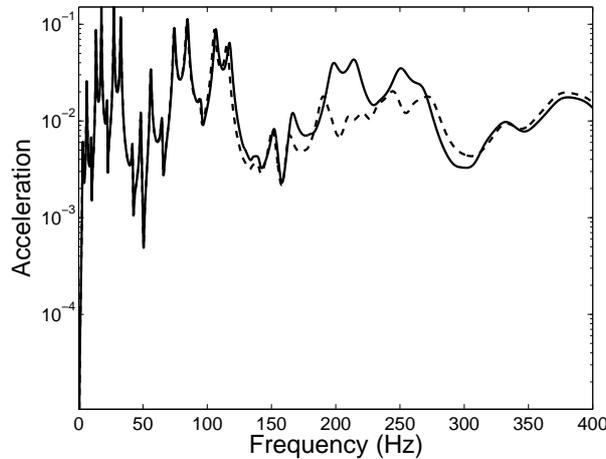
Figure 5: Modulus of the frequency response function of the acceleration in  $x$ -direction at point  $P_{obs}$ : reduced-order computational model (solid line) and reference computational model (dashed line).
