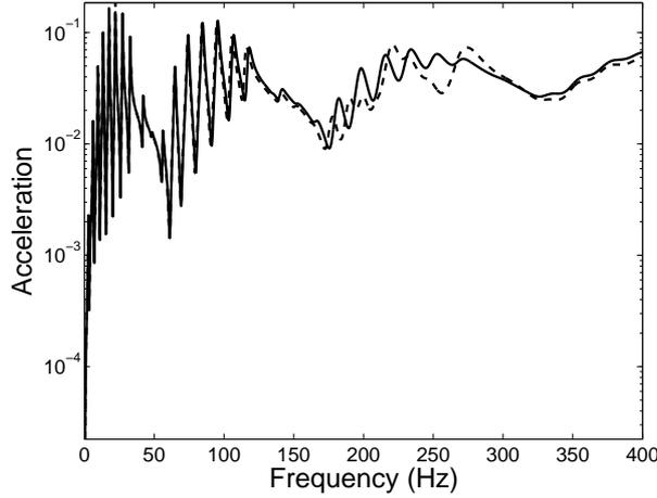
Figure 6: Modulus of the frequency response function of the acceleration in  $x$ -direction at point  $P_{exc}$ : reduced-order computational model (solid line) and reference computational model (dashed line).
