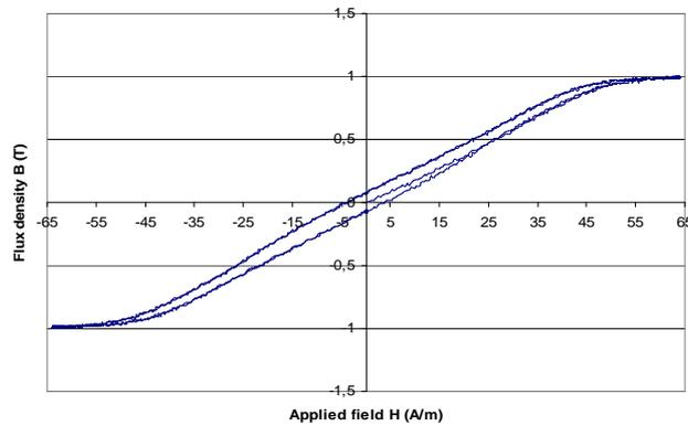
Fig. 4. Flux density as a function of applied field – T=275°C – f=1Hz
