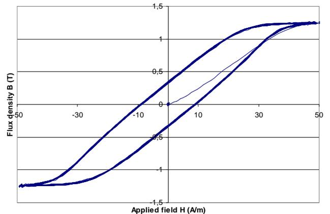
Fig. 2. Flux density as a function of applied field –  $T=75^\circ\text{C}$  –  $f=10\text{kHz}$
