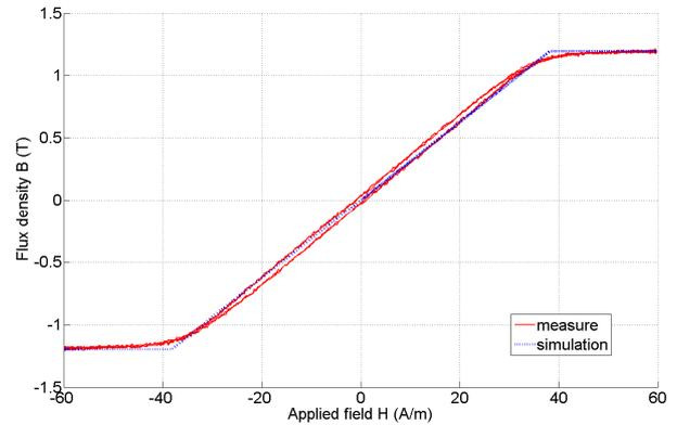
Fig. 5. Measured and simulated B-H curves – T=135°C – f=1Hz
