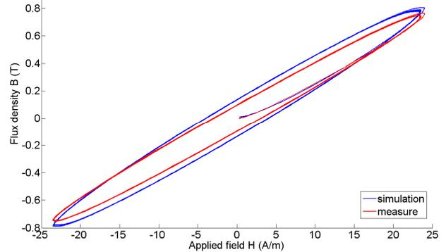
Fig. 6. Measured and simulated minor loops – T=100°C – f=10kHz
