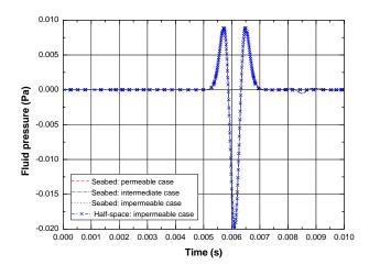
Figure 3: Time evolution of fluid pressure at z=1 cm observation height, for permeable and intermediate ( $\mathcal{K}=5\times10^{-10}~\mathrm{m.s^{-1}.Pa^{-1}}$ ) cases in the seabed configuration, and for impermeable case in both the seabed and the half-space corresponding situation
