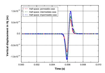
Figure 5: Time evolution of vertical displacement in the half-space corresponding situation to that of Fig. 3
