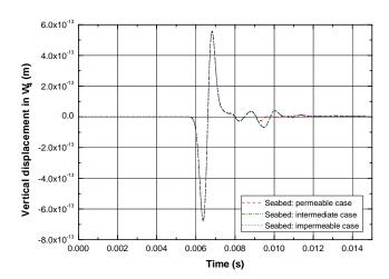
Figure 6: Time evolution of vertical displacement in the fourth layer at z=-80 cm observation height, for permeable, intermediate ( $\mathcal{K}=5\times10^{-10}~\mathrm{m.s^{-1}.Pa^{-1}}$ ) and impermeable cases in the seabed configuration
