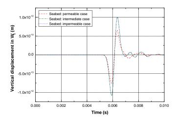
Figure 4: Time evolution of vertical displacement in the first layer at z=-1 cm observation height, for permeable, intermediate ( $\mathcal{K}=5\times10^{-10}~\mathrm{m.s^{-1}.Pa^{-1}}$ ) and impermeable cases in the seabed configuration
