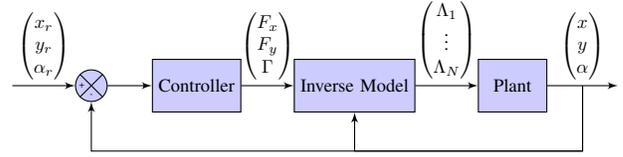
Fig. 2. The inverse modeling control architecture.
