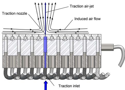
Fig. 5. Cross view of the induced air flow surface showing the generation of the induced air flow (the path of the air flow is darkened).
